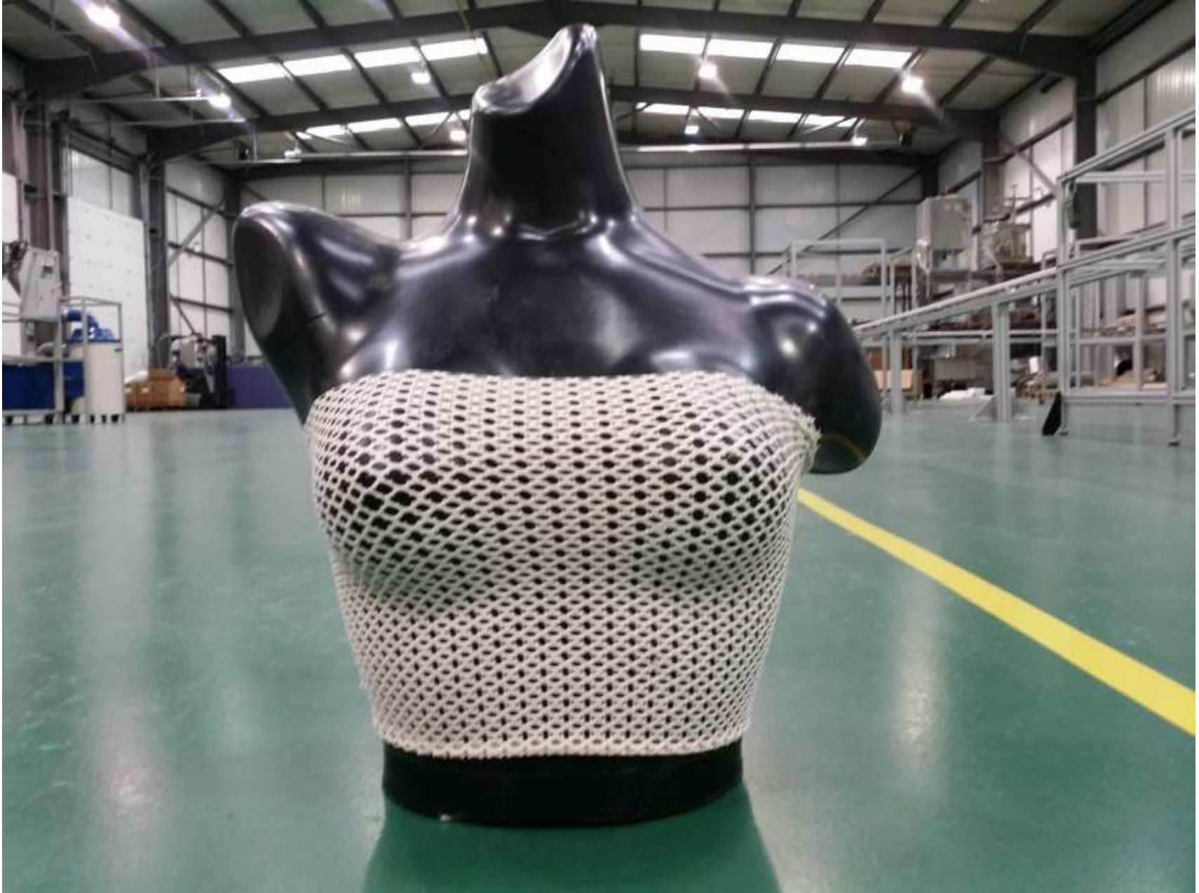
Cosyflex compression wearable garment , made by additive technology to create fabrics
