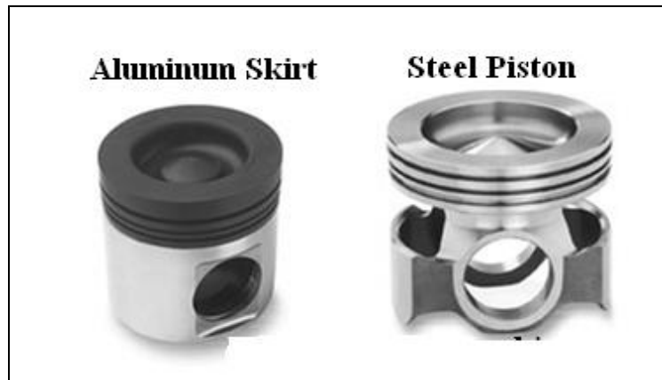
Figure 5.12 Comparison of aluminium and steel piston designs [276].
