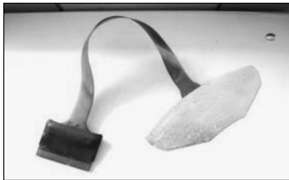
Figure A.1 Pressure sensitive film bonded to metal support plate
