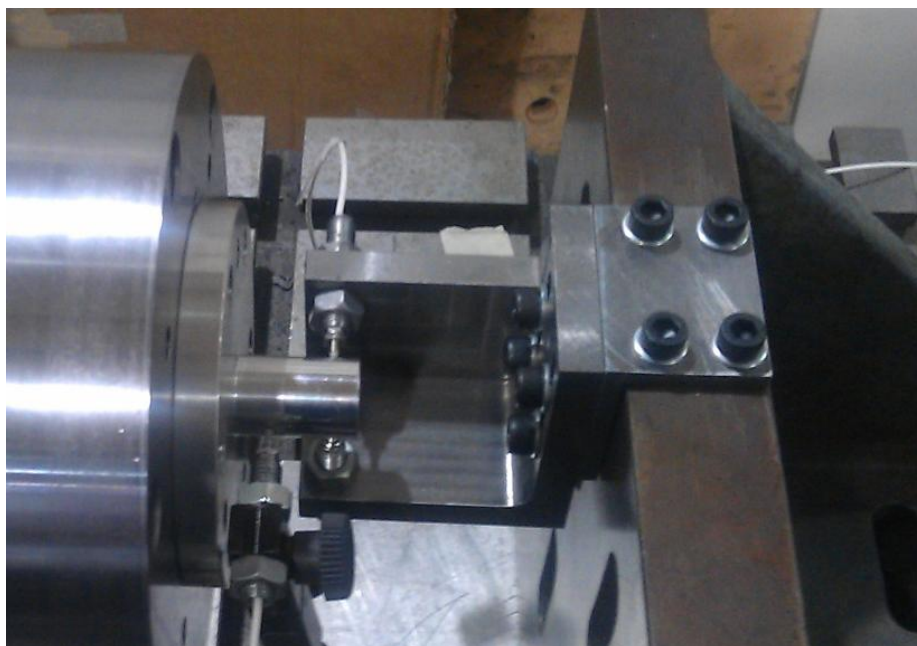
Figure 4.4 – Adjustable fixture of radial error motion testing
