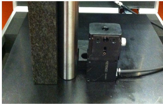
Figure 3.7 – Static resolution test setup
