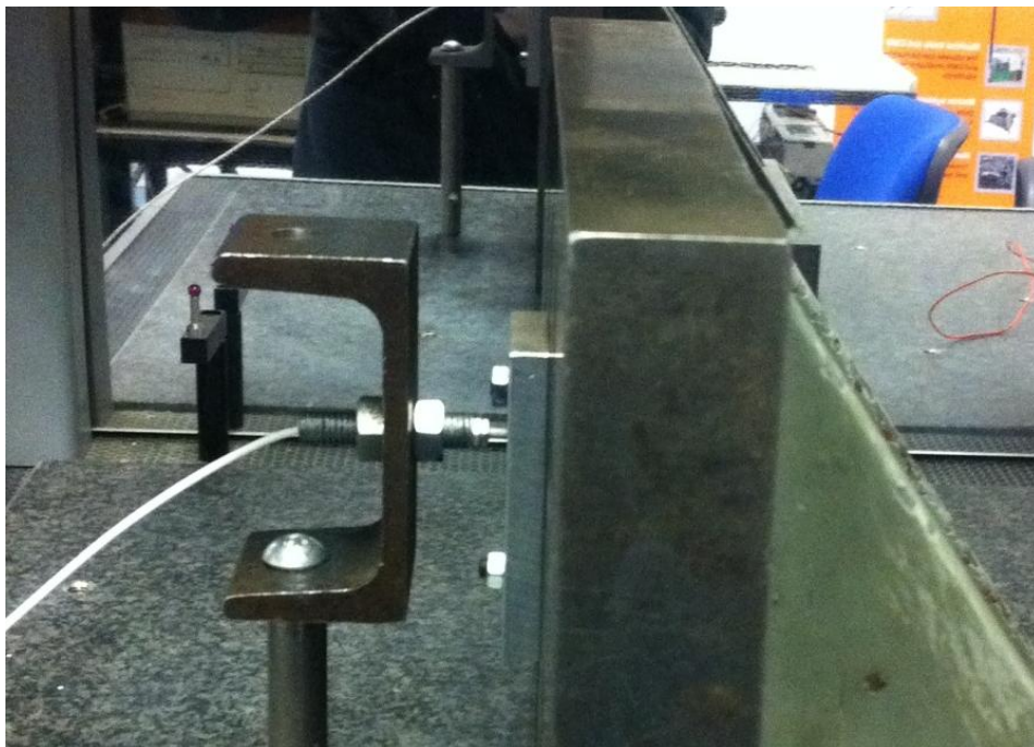
Figure 3.22 – Eddy current static resolution test setup
