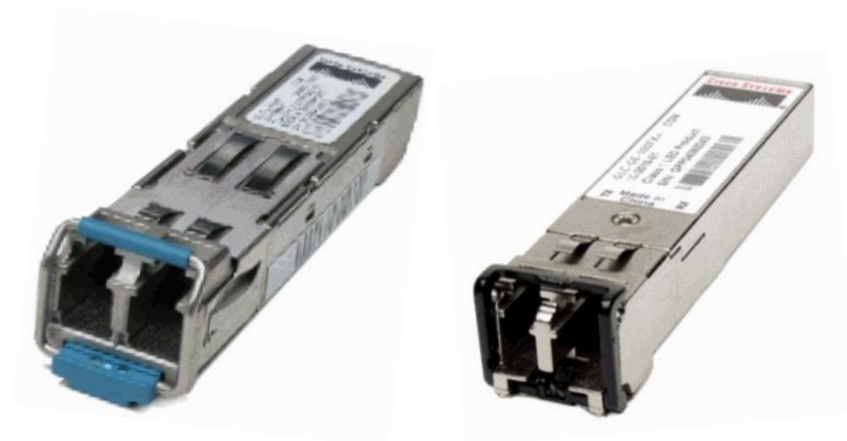
Figure 25: SFP+ module for fibre channel (left) and SFP for Gigabit Ethernet
