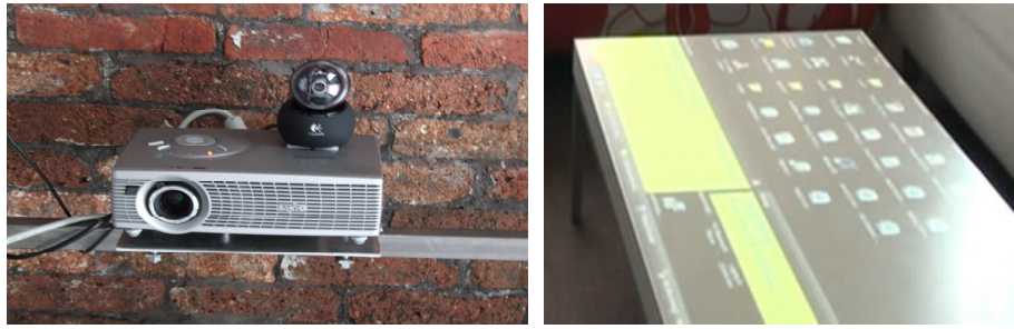
Figure 5.2: The projector (left) rendered interfaces on the coffee table (right)
