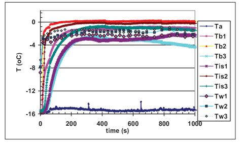
**Figure 1**. Typical plot of the temperatures measured by thermocouples and IR camera during the experiment with a small channel and  $V_a=20 \text{ m s}^{-1}$ :  $T_{a}$ - air temperature;  $T_{b}$ -temperature of bottom of the channel;  $T_{is}$ -ice surface temperature;  $T_{w}$ - temperature of the surface of flowing water measured by IR camera. 1.,2. and 3. designate chosen sites.
