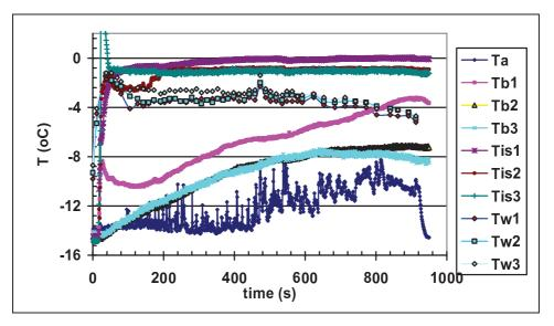
**Figure 2**. Typical plot of the temperatures measured by thermocouples and IR camera during the experiment with a large channel and  $V_a=30 \text{ ms}^{-1}$ :  $T_a$ - air temperature;  $T_b$ -temperature of the bottom of channel;  $T_{is}$ -ice surface temperature;  $T_w$ - temperature of the surface of flowing water measured by IR camera. 1.,2. and 3. designate chosen sites.
