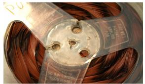
Fig.1: a tape affected by severe curly tape deformation.
