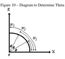
The preliminary samples utilising a conventional yarn found that a six-segment hemisphere produced the smoothest curve when the radius was calculated to be 7.5 cm. It was thus decided to investigate a series of sizes of hemispheres using the nylon covered carbon yarn. Equation 1 was utilised to determine the appropriate measurement for each segment division to enable a knitting plan to be produced. The sizes of hemispheres were calculated to achieve diameters of 15, 16, 17, 18, 19, 20 and 25 cm.
