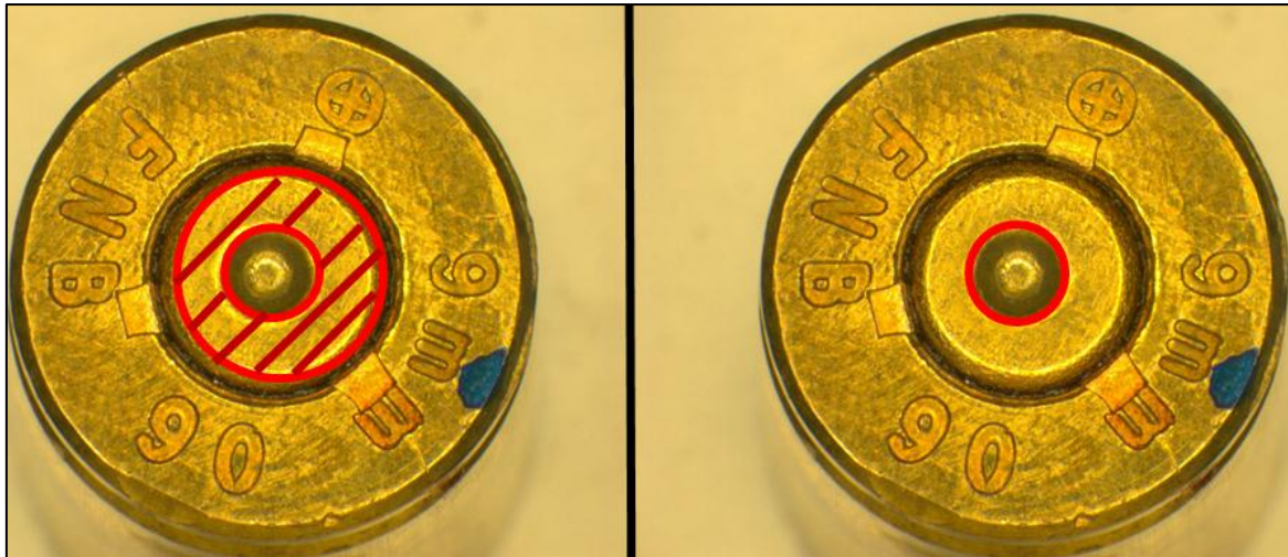
Figure 2-13: Cartridge Case Head with Breech Face Impression (Left) and Firing Pin Impression (Right)
