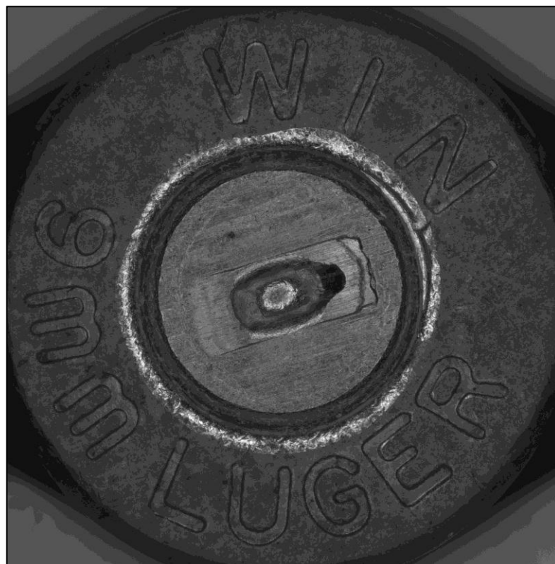
Figure 2-14: A Cartridge Case Head Showing the Class Characteristic of a Rectangular Firing Pin only Produced by Glock Weapons
