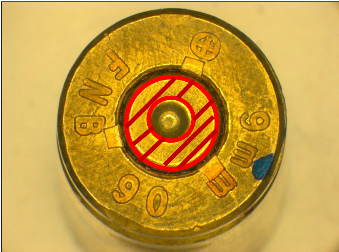
Figure 5-3: Cartridge Case Head Showing the Breech Face Impression (Area Between the Two Red Circles).
