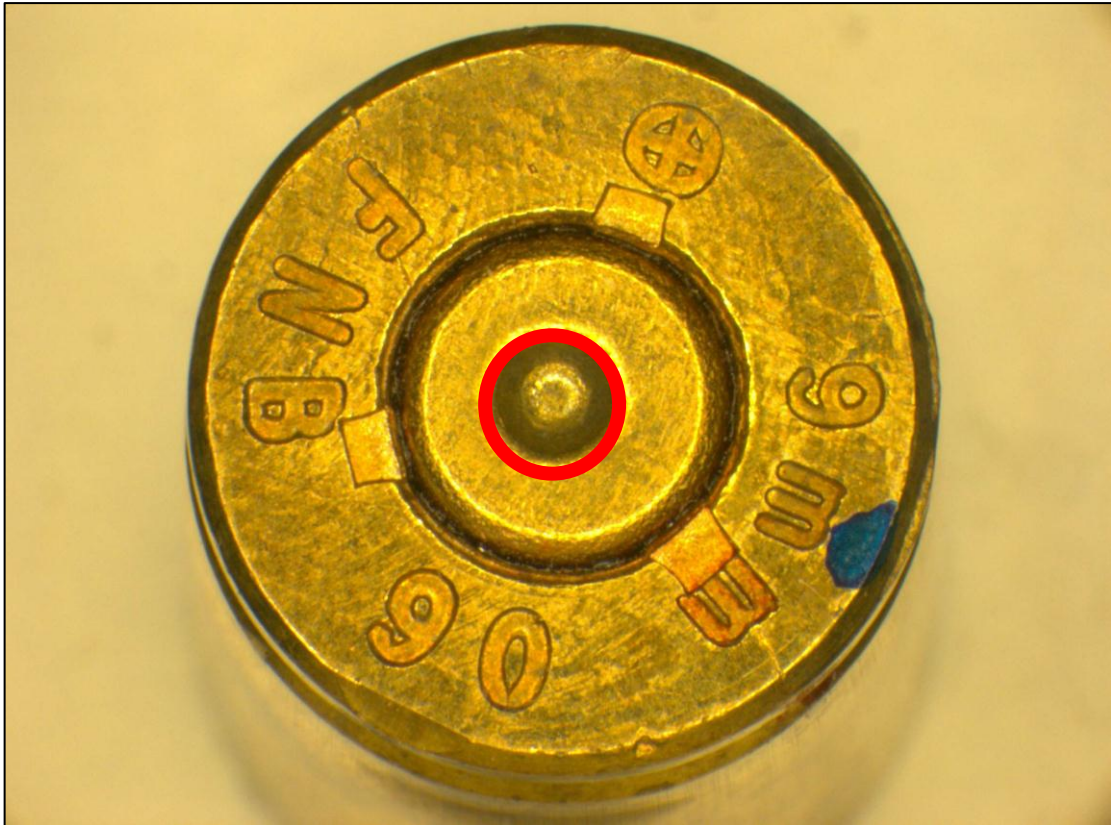
Figure 5-4: Cartridge case Head with Firing Pin impression Marked (Area inside the Red Circle)
