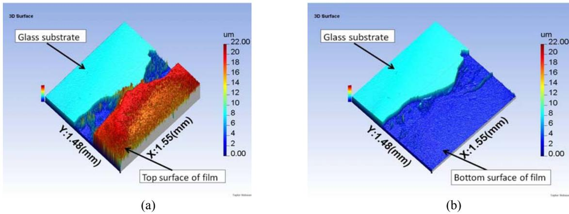
Fig. 3. measurement data from one area showing (a) top surface of the film and glass substrate; (b) bottom surface of the film and the glass substrate.
