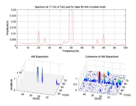
Figure 7 Spectrum and bispectrum at 77.3% of full load for gear with broken tooth
