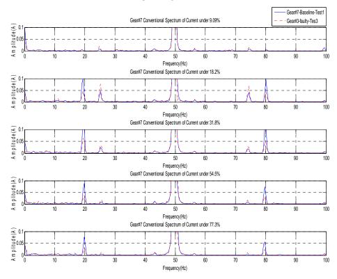
Figure 4 Motor current signals in non-slip compensation mode
