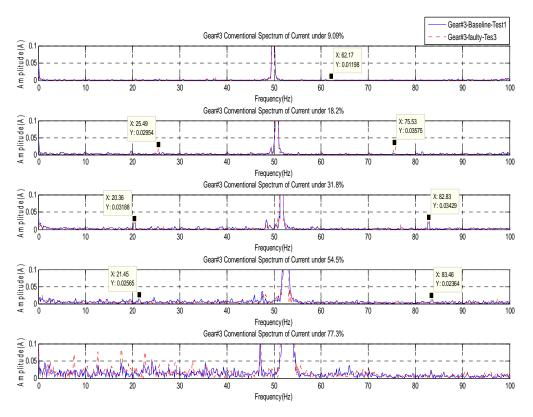
Figure 5 Motor current signals in slip compensation mode
