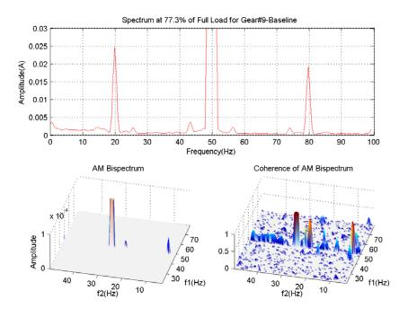
Figure 6 Spectrum and bispectrum at 77.3% of full load for healthy gear
