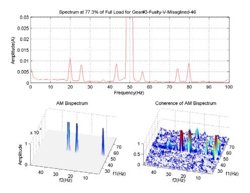
Figure 8 Spectrum and bispectrum at 77.3% of full load for gear with broken tooth and 0.46mm misalignment
