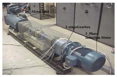
Figure 1 Test rig construction
