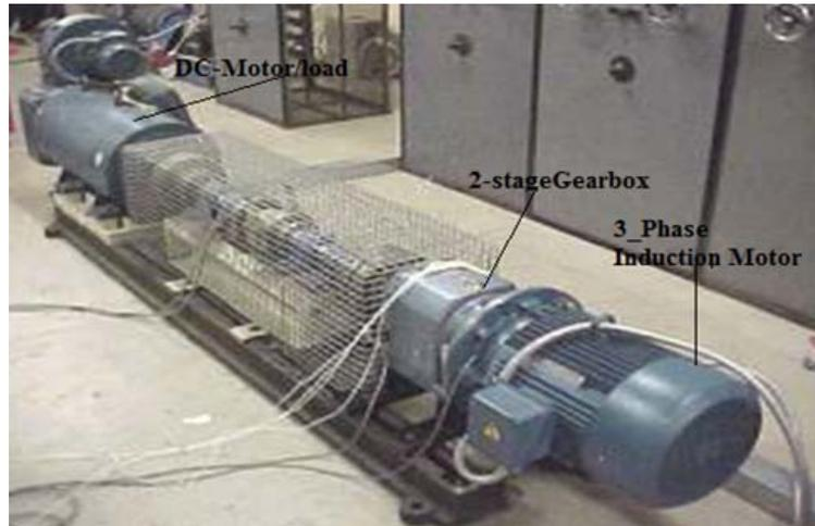
Figure 1 Test rig construction
