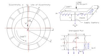
Figure 2 Dual Hole Entry Hybrid Bearing
