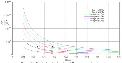
Figure 3.1 Graph showing bearing stiffness against bearing gap
