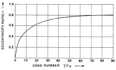
Figure 4 Lubrication Theory Design Chart[4] showing Load Number against Eccentricity Ratio
