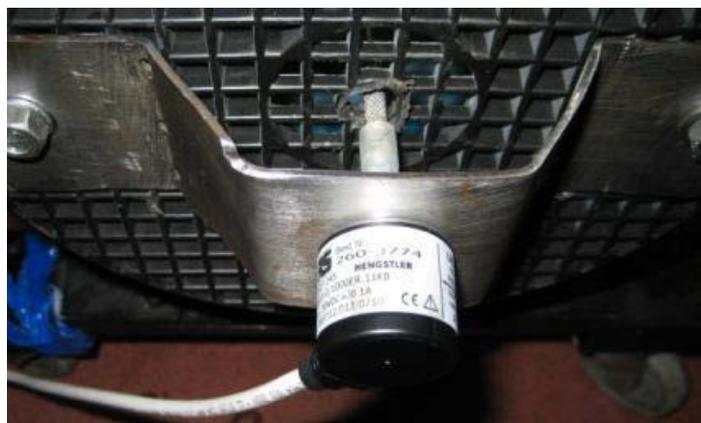
**Figure 7-2 - Mounting of motor encoder**
