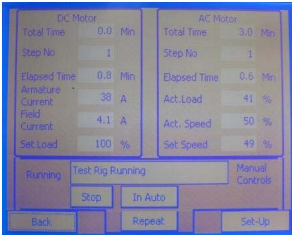
Figure C-23 - Operator Screen; Test Rig running in Auto
